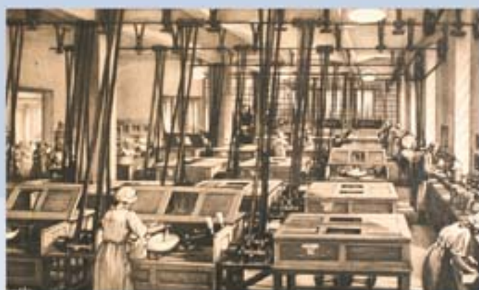
[36] Trituration machines of the Willmar Schwabe Company, Leipzig, c. 1924
